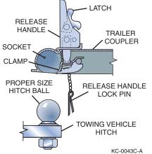
Trailer hitch balls are sized and rated for use based on the trailer GVWR:
