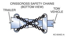
chains under the trailer tongue to prevent the tongue from dropping to the road if the trailer separates from the hitch ball. Rig the chains as tight as possible with enough slack to permit full-free turning. Safety chains must be rated at the same or greater weight capacity as the trailer's GVWR.
