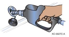
you to manually turn the fuel valve, while the antisiphon valve operates automatically. Because gasoline fumes are heavier than air, they will sink to the lowest part of your boat, such as the bilge. Always evacuate fumes with the bilge blower (if equipped) before attempting to start the engine.
