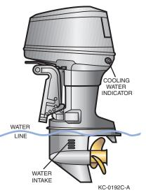
engine's cooling system is operating properly.
