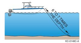
plenty of additional anchor line on board. If anchoring in tidal waters, consider a rode chain about the length of the boat and increase the total anchor line length to ten times the depth of the water at low tide.
