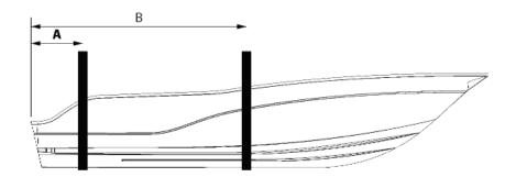
A- AFT SLING LOCATION PORT AND STARBOARD
