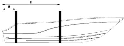
A- AFT SLING LOCATION PORT AND STARBOARD (28")
