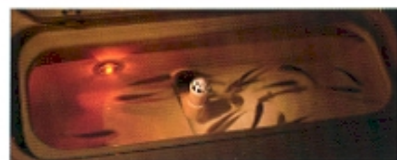
Standard aerated, lighted 33-gallon live well | 12v
