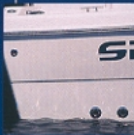
Tournament Package Stainless Rub Rail, Chrome Over Brass Thru-Hull Fittings
