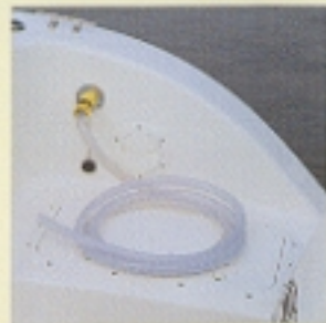
230 CC standard raw water wash down
