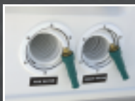
Fresh & raw water hydracoil hoses & sprayheads
